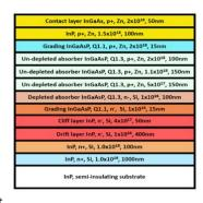
Epitaxial layer configuration of InGaAsP/InP photodiode. Drawn from Ref [1].
