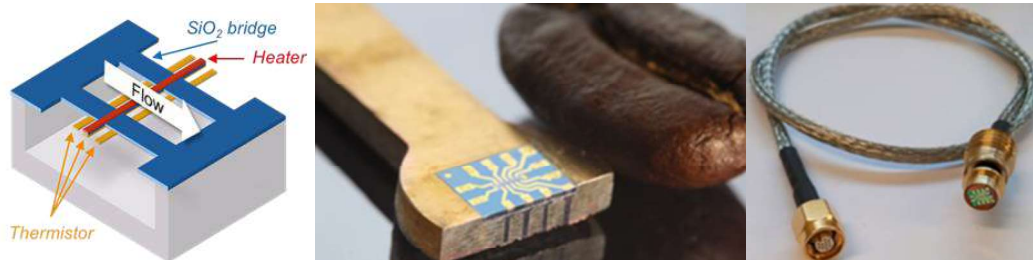
FIGURE 2: HTGS calorimeter wall shear stress design (left). Flush mounted device with Through Silicon Vias (middle). Coaxial integration of the HTGS sensor (right).
