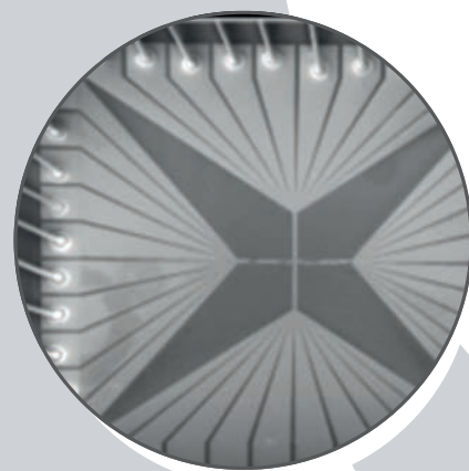
Micro-solder in ball mode on a crossbar device 100nm
