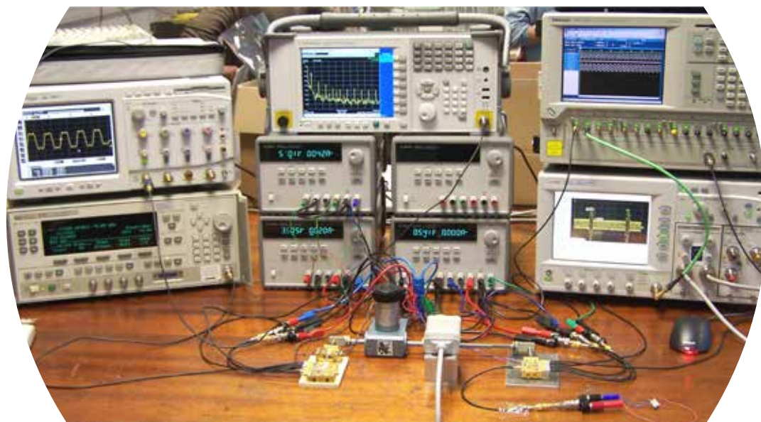
Mixed signal test bench for an UWB-IR communication system operating at 60 GHz
