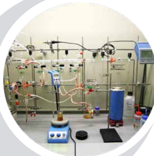
Vacuum / nitrogen manifold
