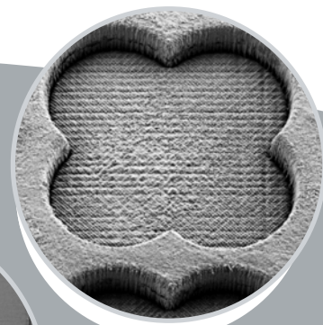
AlN micromachining : Blind and pass-through via (nanosecond laser system)
