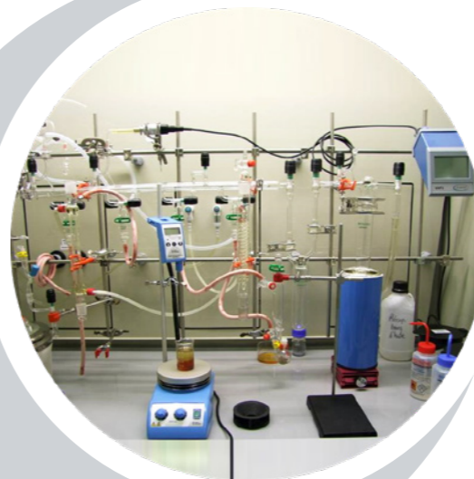
Vacuum / nitrogen manifold
