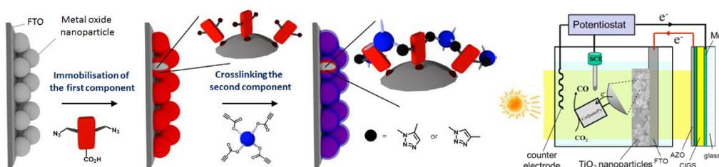
*Figure. Schematic representation of the copper free click chemistry methodology to crosslink the dyes over a mesoporous film (left) and of a CIGS based photocathode (right).*
