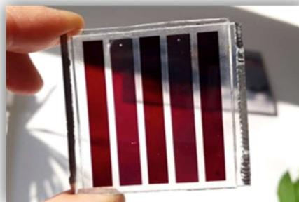
Figure 1: Mini-module (active surface area: 14 cm<sup>2</sup>) prepared with an organic dye synthesized in this work.
