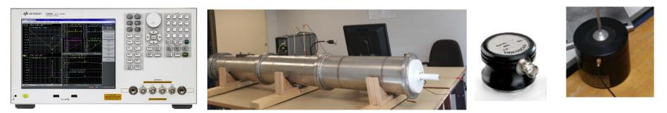
Oscilloscopes, network /impedance analyzer, power supplies, signal generators, generators, developed specific Kundt Tube ...
