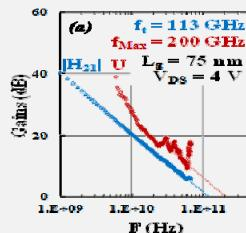
Current gain and cut-off frequency of a  $2 \times 50 \times 0.225\mu\text{m}^2$  InAlN/AlN/GaN HEMT
