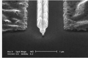
SEM view of the cross section of double-T-shaped gates
