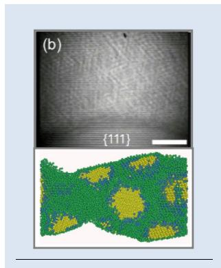
All-atom molecular dynamics simulation of a superplastically deformed poly-Si nanostructure, at 20-fold elongation. Above, experimental TEM image of a MEMS nanocontact which inspired the computer simulation (Cnrs-LIMMS Tokyo).
