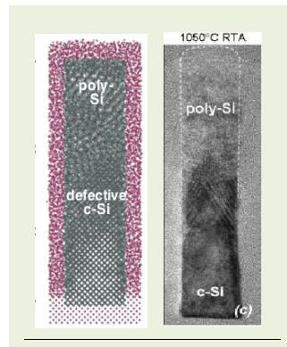
Molecular dynamics simulations of a FinFET device (Philips) to study the dynamical growth of the Si/oxyde interface. On the right, experimental TEM image after thermal annealing.
