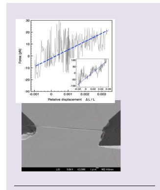
Molecular dynamics simulations of a stretched DNA artificial structure, and its stress-strain plot for estimating Young's modulus. Bottom: SEM micrograph (Cnrs-LIMMS Tokyo) of a DNA bundle stretched between the tips of MEMS nanotweezers.
