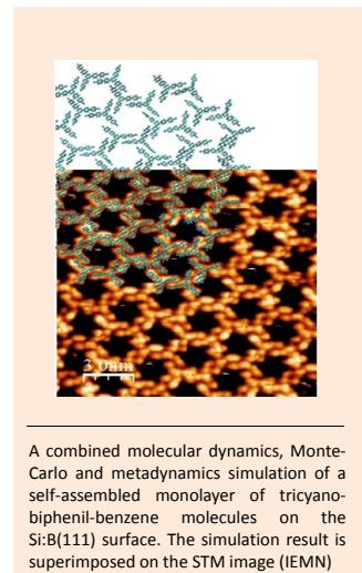
A combined molecular dynamics, Monte-Carlo and metadynamics simulation of a self-assembled monolayer of tricyanobiphenyl-benzene molecules on the Si:B(111) surface. The simulation result is superimposed on the STM image (IEMN).
