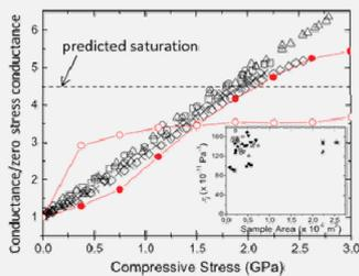
Piezoresistance in bulk p-type (110) silicon in compression up to 3 GPa.<sup>(3)</sup>
