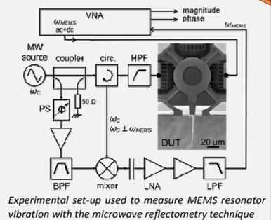
Experimental set-up used to measure MEMS resonator vibration with the microwave reflectometry technique
