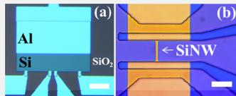
4 terminal aluminium-silicon hybrid structure fabricated at IEMN which displays giant piezoresistance<sup>(1)</sup>. Scale bar = 20  $\mu\text{m}$ . (b) Top-down silicon nanowire<sup>(2)</sup> fabricated at IEMN used for giant piezoresistance studies. Scale bar = 2  $\mu\text{m}$ .
