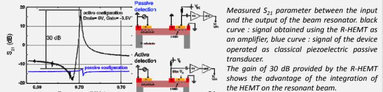
Measured  $S_{21}$  parameter between the input and the output of the beam resonator. black curve : signal obtained using the R-HEMT as an amplifier, blue curve : signal of the device operated as classical piezoelectric passive transducer. The gain of 30 dB provided by the R-HEMT shows the advantage of the integration of the HEMT on the resonant beam.
