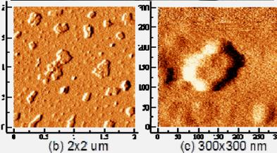
(a) SEM image of a MEMS AFM sensor based on a silicon ring resonator. Vibration is driven and sensed by integrated capacitive transducers featuring sub-100 nm air gaps. A silicon nanotip (apex radius below 10 nm) is located at a maximum of the elliptic vibration mode. (b) and (c): AFM topographic images of DNA origamis acquired by a 10.9 MHz MEMS AFM sensor. AFM tip vibration amplitude is 0.2 nm.
