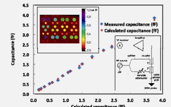
Main: comparison between the calculated and measured capacitance values. insets: microwave interferometer and capacitance image obtained after calibration.
